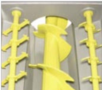
Feeding device wood crusher
