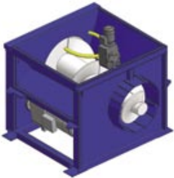
Screw Compactor with whirler Fractions: paper, cardboard, small cardboard packaging
