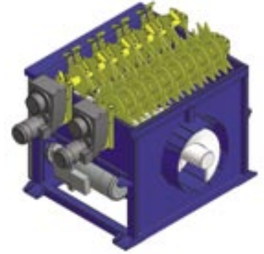
Cardboard pre-crusher Fractions: heavy duty cardboard and flat cardboard packaging for automatic loading
